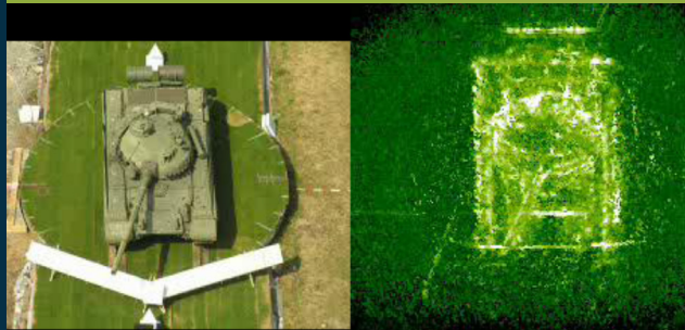
SET-172: An example of a radar image of a tank obtained from turntable measurements.
